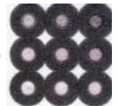
Hydrophilic area for colorimetric detection
